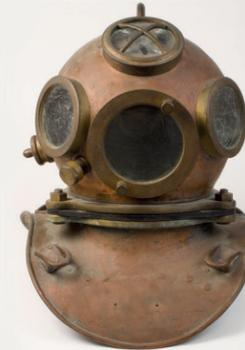
The helmet is made of heavy bronze with thick glass windows for the diver to look out of. Air for breathing was provided through an attached hose.
